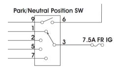
Example of a serial switch. One common wire will switch to each individual position in series.
