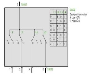
Example of a parallel switch. One common wire will switch to multiple position in paralel creating a binary code combination.
